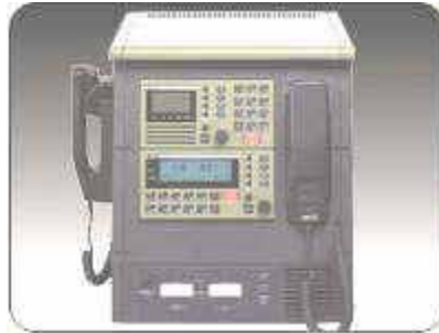
Typical GMDSS A2 station
