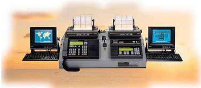
Typical GMDSS A3 station
