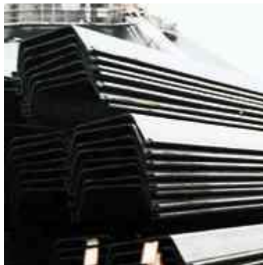
No. 26 Sheet pilings ready for shipment
