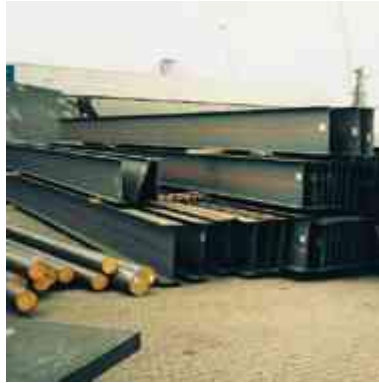
No. 11 Structurals: hot rolled steel beams or joists stored on the open quay
