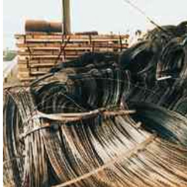
No. 25 Wire rods: disintegration of bundles caused by bad stowage & rough handling
