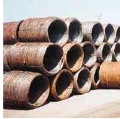
No. 14 Hot rolled wire rods: no wrappers (unprotected) stored in the open air
