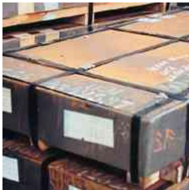
No. 8 Cold rolled steel sheeting in packages
