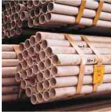
No. 12 Pipes correctly bundled and strapped
