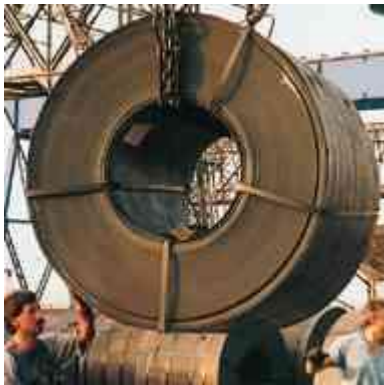
No. 1 Hot rolled steel coil provided with steel channels to prevent edge damage.
