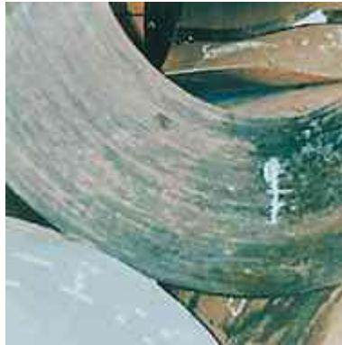
No. 21 Silver nitrate. Note milky white area: positive reaction
