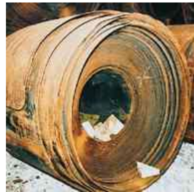
No. 23 Hot rolling coils - excessive telescoping
