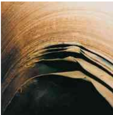
No. 22 Hot rolled coils. Note bending damage to inner circumference turns of plating
