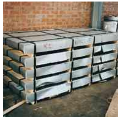
No. 9 Cold rolled steel sheeting in packages
