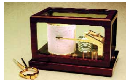
The barograph (above) records readings, allowing you to keep an eye on trends; the electronic barometer (left) does the same thing
